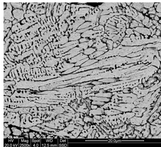
Fig. 8 BSE images showing microstructures of a laser fabricated sample at scan speed of 20 mm/s, laser power of 100 W, scan interval of 0.05 mm, and layer thickness of 0.05 mm
